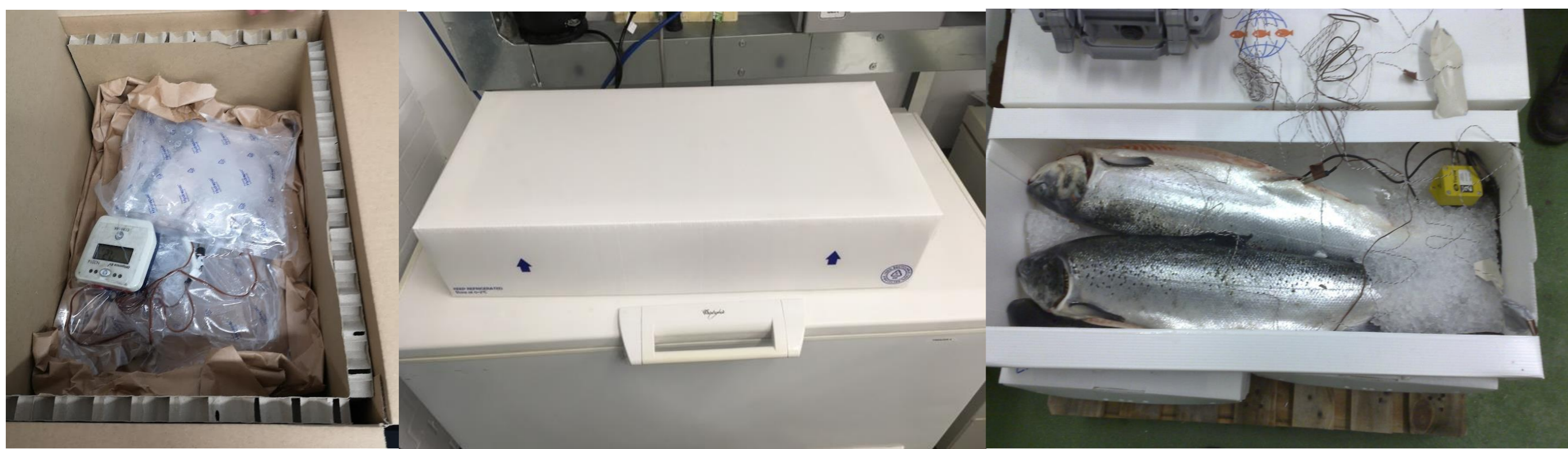
Examples of box packaging materials tested: corrugated cardboard, polypropylene, and a secondary polypropylene multilayered box.
