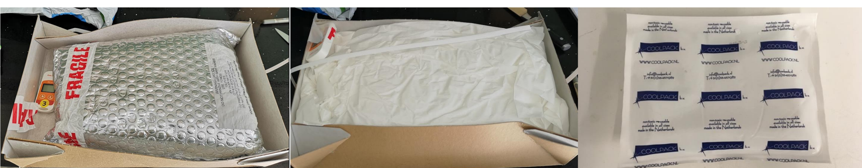
Examples of insulative materials and cold packs tested: Foil-coated bubble wrap, paper wrap, frozen gel pack.
